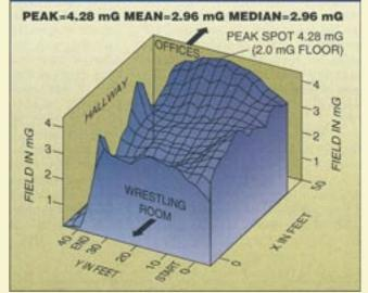
After shielding, magnetic field readings dropped to a mean level 2.96 mG from 34.5 mG before shielding. Peak levls dropped to 4.28 mG from 111 mG.
