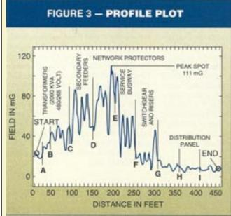
A profile plot shows magnetic field readings along the path taken by surveyors, shown in Fig. 2. Letters correlate to turn markers in Fig. 2.
