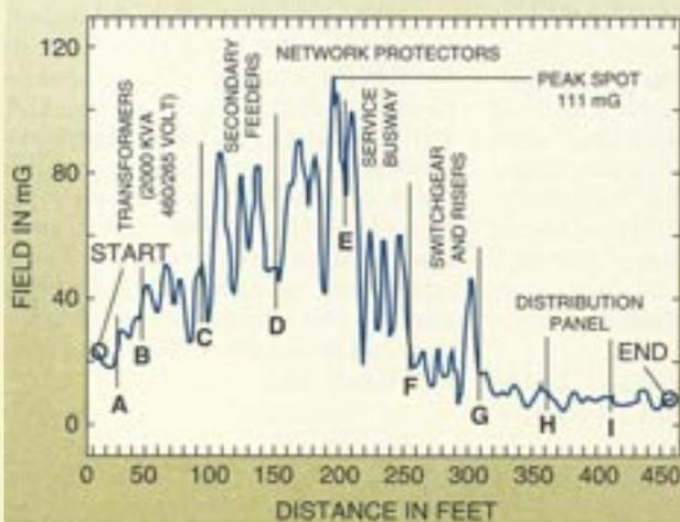
A profile plot shows magnetic field readings along the path taken by surveyors, shown in Fig. 2. Letters correlate to turn markers in Fig. 2.
