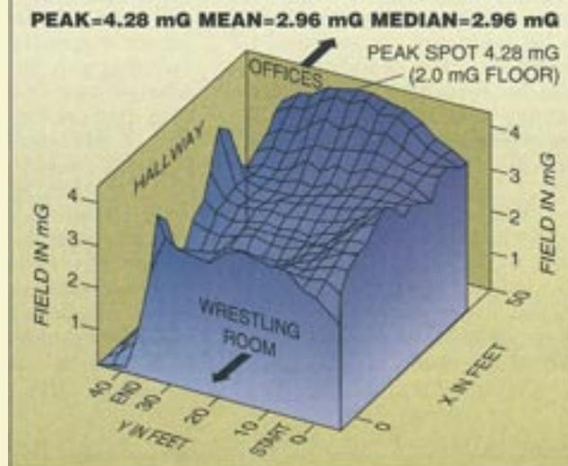
After shielding, magnetic field readings dropped to a mean level 2.96 mG from 34.5 mG before shielding. Peak levels dropped to 4.28 mG from 111 mG.
