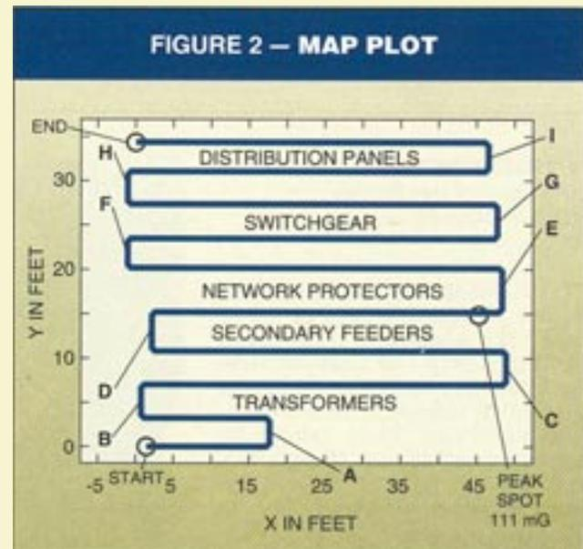
Superimposing the path taken by surveyors over a map showing equipment in the space below helps identify key areas contributing to high magnetic field readings.
