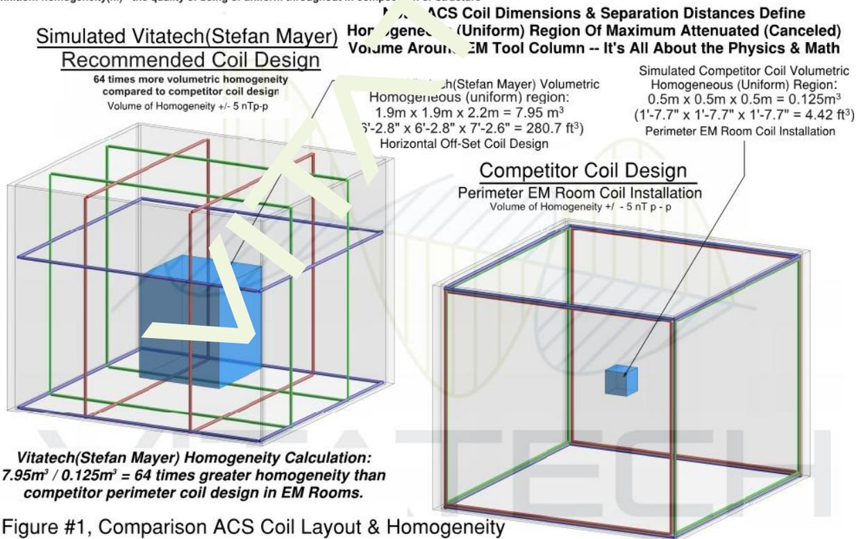
Figure #1, Comparison ACS Coil Layout & Homogeneity
